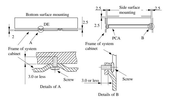
Figure 3.3 Mounting frame structure
